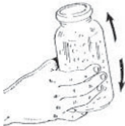
Figure 19: The ‘salt method’ of checking grain moisture content
